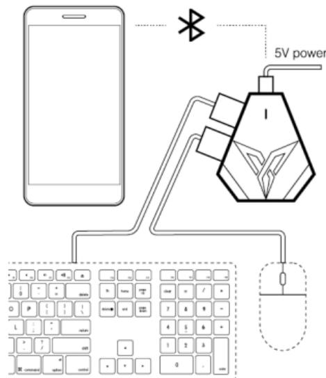
Note: keyboard/mouse extension supports USB keyboard and mouse devices, including USB wired keyboard and mouse, wireless keyboard and mouse suite and wireless mouse
